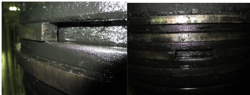
Figure 2. Damaged piston rings
